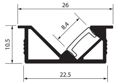
Each metre of fossLED profile comes with two End Caps (one with and one without a cable feed hole) as standard; for extra accessory packs please quote code PRO6R-OAC.
